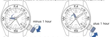
Turning the crown slowly, checking that the hour hand moves in one-hour incre When adjusting the hour hand, the other hands may move slightly. Ho ver this is not a malfunction 6 Push the crown in.
