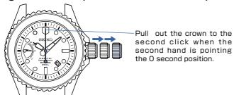
$oldsymbol{3}$  Turn the crown in the direction shown by the arrow to set the time.
