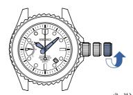
4 Push the crown back in to the normal position in accordance with a time signal.
